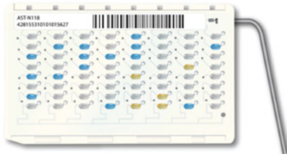
FIGURE 3. Vitek 2 antimicrobial susceptibility testing card (bioMérieux)
